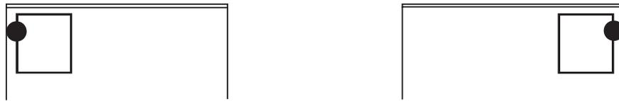
The back half of the dot is attached to the bracket with a #8-32 x 5/8" flat head screw. A 3/32" allen wrench (provided) is required to loosen or tighten the screw. The dot can rotate with this screw loose to position the plaque.
