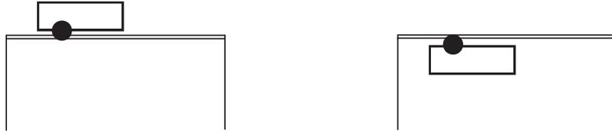
**SIDE PANEL:** Bracket clips into the slots of the hanger frame. A #6 x 1/2" pan head screw (provided) secures the bracket to the panel and prevents the bracket from "hinging". Do not drill a hole. Use a screw driver and the hole in the bracket as a template to align and fasten the screw through the fabric into the fiber board at the side of the panel.
