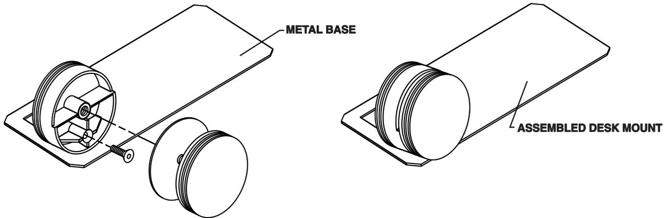
The back half of the dot is attached to the bracket with a #8-32 x 5/8" flat head screw. A 3/32" allen wrench (provided) is required to tighten the screw if necessary. The screw holding the back half of the dot to the bracket **must be firmly tightened** to hold the dot and the plaque in upright position.
